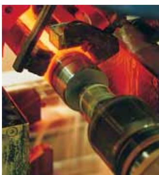
▼ Shaft induction hardening
